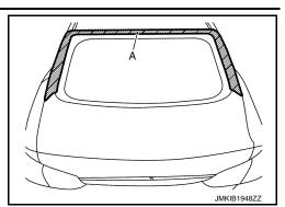
7. Paint matching marks on the rear window glass and body panel, positioning during installation can be easily performed.
