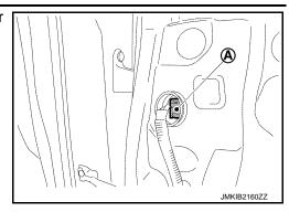
3. Remove rear door regulator assembly mounting bolts (A) and nuts (B).
