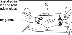
10. Use suction lifter (A) or rubber suction cups that are installed in advance, align the matching marks between the holder and roof panel hole and between the body panel and rear window glass
