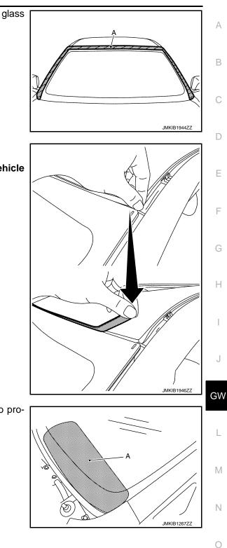
16. Remove windshield glass upper molding. CAUTION: Remove windshield glass upper molding left on vehicle
