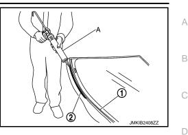
Use suction lifter (A) or rubber suction cups that are installed in advance, align the matching marks between the holder and roof panel hole and between the body and windshield glass (1) to install them on the vehicle.
