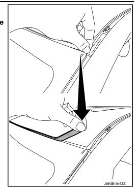
18. Apply protective standish cover (A) on instrument panel to protect it from damage.
