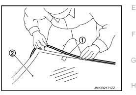
7. Apply primer for glass along the entire circumference of rear window glass. Use the sealing kit for glass application and the special holder for cartridge or similar tools. CAUTION: There are 2 to man of primer. Never confuse the application methods.
