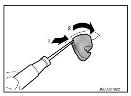
Peel off dual lock fasteners (A) between headlining assembly and roof panel. (With sunroof) CAUTION: Never bend headlining when removing.
