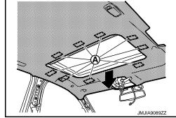
12. Remove front portion of headlining as shown in the figure. **CAUTION:**
