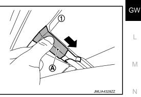
b. Disengage inside miror harness cover fixing pawls, and then remove inside miror harness cover.
