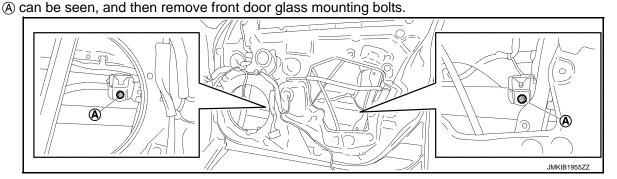
Hold securely front door glass and pull it out of front door panel to remove front door glass. CAUTION:
