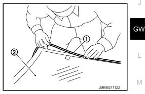
7. Apply primer for glass along the entire circumference of rear window glass. Use the sealing kit for glass application and the special holder for cartridge or similar tools.
