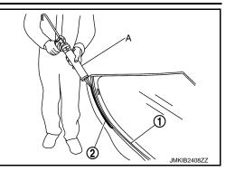
11. Use suction lifter (A) or rubber suction cups that are installed in advance, align the matching marks between the holder and roof panel hole and between the body and windshield glass (1) to install them on the vehicle.
