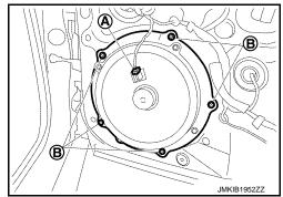
4. Remove front door inner frame mounting bolts (A) and fixing clips (B), and then remove front door inner frame.
