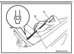
b. Tie both ends of the piano wire (B) to the wire grip (A), etc.
