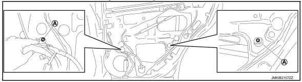
12. Hold securely rear door glass and pull it out of rear door panel to remove rear door glass.
