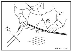
Apply primer for glass along the entire circumference of glass. Use the sealing kit for glass application and the special holder for cartridge or similar tools. CAUTION:
