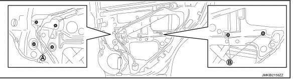
4. Remove rear door regulator assembly according to numerical order 1→3 indicated by arrows as shown in the figure, and then remove rear door regulator assembly.
