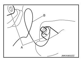
Use suction lifter (A) or rubber suction cups, etc. to remove rear window glass from the vehicle.
