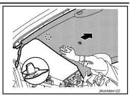
6. Apply protective tape (A) on body panel around rear window glass to protect painted surface from damage.
