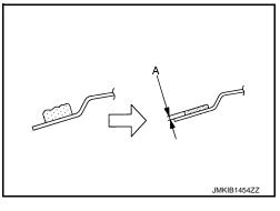
2. Remove remaining adhesive ① and sealant using a cutter (A) smooth out rear window glass surface ②.
