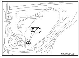
6. Peel off rear door sealing screen using a cutter-knife (A).
