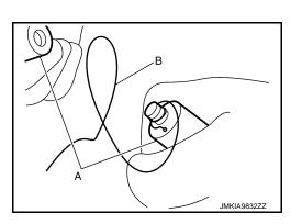
Using a windshield cutter (A) into the bonded area. Cut the adhesive by pulling the knife, keeping the tip parallel to the edge of glass.
