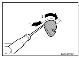
Peel off dual lock fasteners
